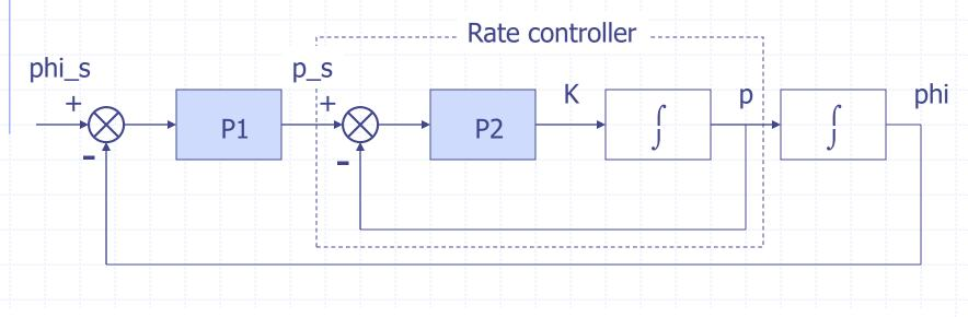
Cascaded P Controller: stable (for not too high P1 and P2! and P2 >> P1)
