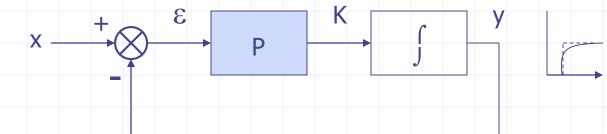
$\begin{aligned} Y(s) &= P H(s) (X(s) - Y(s)) \\ Y(s) &= (P H(s) / (1 + P H(s))) X(s) = H_{PC}(s) X(s) \end{aligned}$
