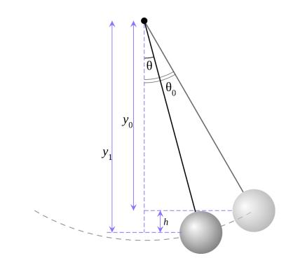
Think of a pendulum. If the setpoint is hanging straight down, then gravity acts as a proportional controller for the position... Pendulum will oscillate!
