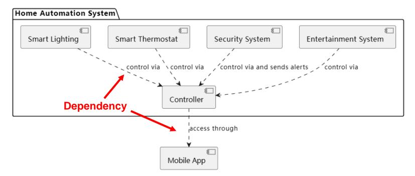
• **Component:** represents a modular part of a system that encapsulates its contents.
